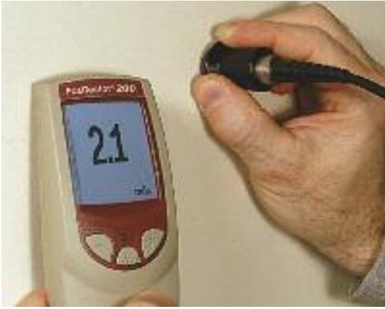
An ultrasonic instrument being used to measure on textured surfaces.
